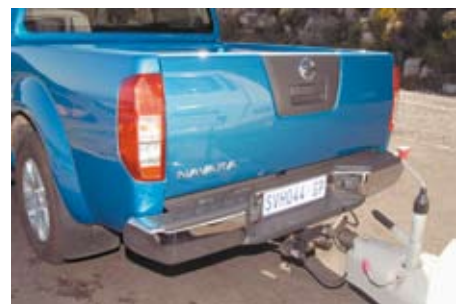
Lower than a standard 4x4 the Navara does away with needing a drop plate for the correct tow-ball height.
