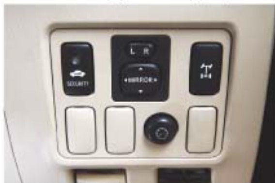
... electric rear diff lock for when you need more than conventional 4x4 traction...
