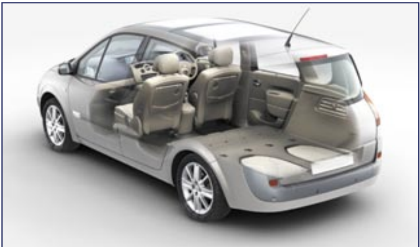
Above, a schematic diagram shows the seven seater layout and below, the seats folded flat. Seats can be folded one at a time depending on the need for space.
