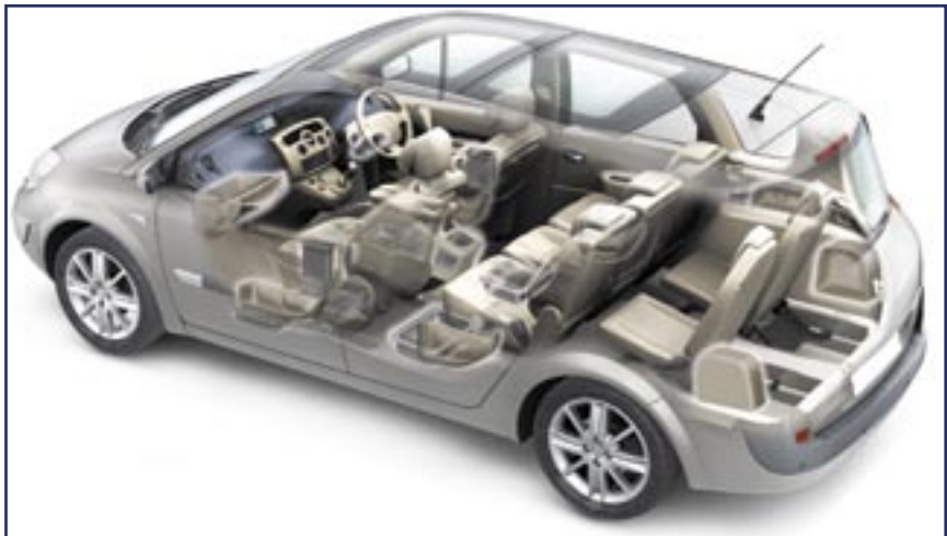
Above, a schematic diagram shows the seven seater layout and below, the seats folded flat. Seats can be folded one at a time depending on the need for space.
