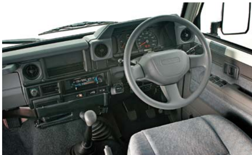
Dashboard layout is simple and functional; note the diff-lock just below the steering wheel on the left.
