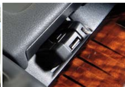
Depressing a button with the key inserted starts the car.
