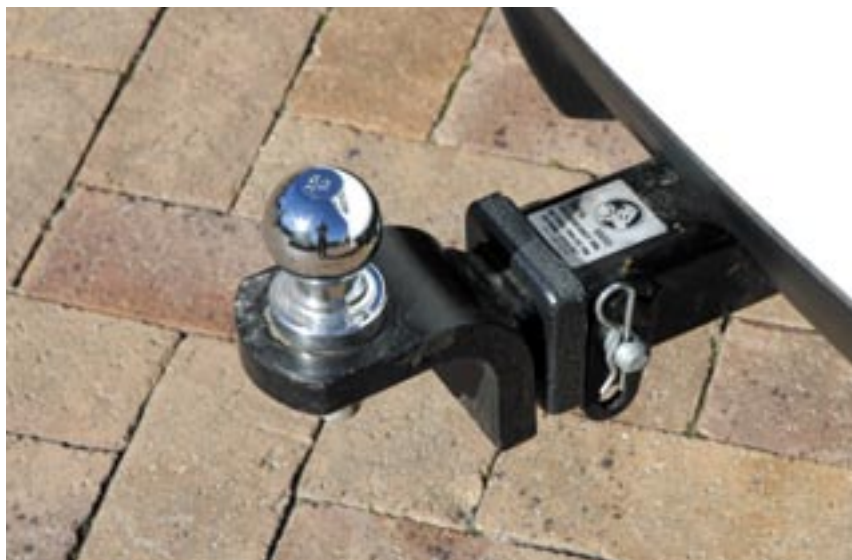
The detachable factory-fitted towbar (just pull the pin!) may offer new challenges for stabiliser manufacturers but the interesting point is the electrical socket. It's on the end of a harness found inside the boot.
